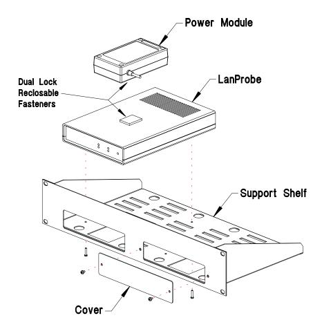
Figure 3-11: Installing LanProbe in the Rack Support Shelf
